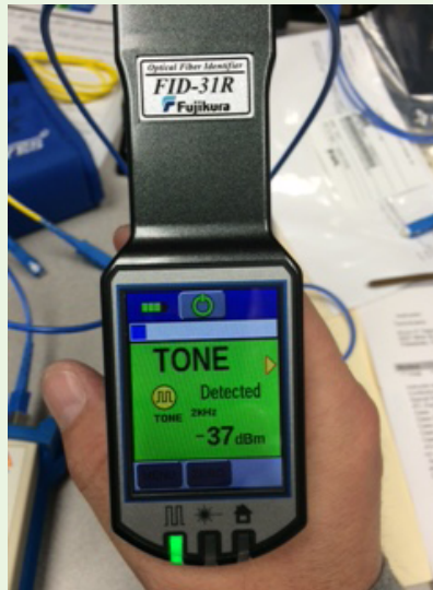
Tested on G.657B bend insensitive OFS SM fiber with blue 900-µm buffer and 2-mm blue PVC jacket
