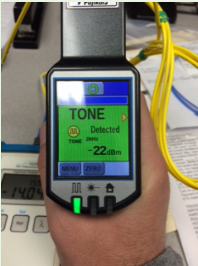
Tested on Fujikura G.652D SM fiber with blue 900-µm buffer in a 2-mm yellow PVC jacket
